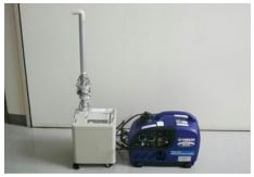
Portable dust iodine sampler
