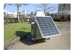
Portable monitoring post with PV generator and cellular phone communication function
