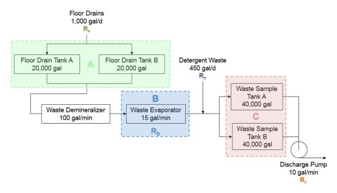
Figure 3-29 Example of liquid waste processing system flow stream scheme
