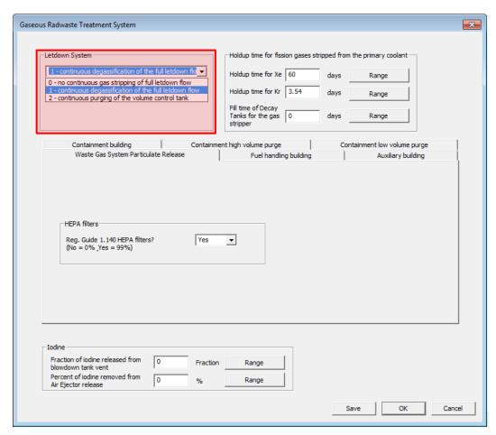
Figure 3-54 Gaseous Radwaste Treatment System Screen with Letdown System field options
