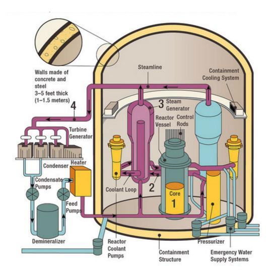
Figure 3-9 Basic structure of a PWR
