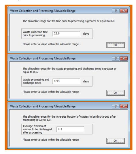
Figure 3-26 Waste Collection and Processing Allowable Range Screens
