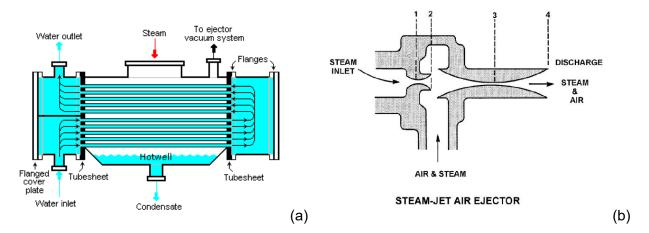
Figure 3-61 Diagram of turbine condenser (a) and steam-jet air ejector (b)
