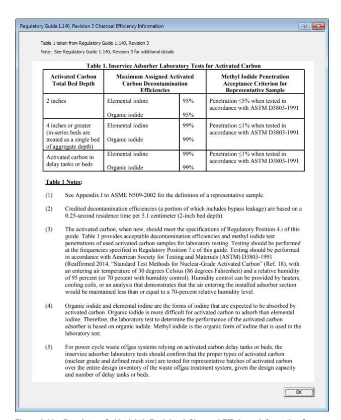
Figure 3-66 Regulatory Guide 1.140, Revision 3 Charcoal Efficiency Information Screen
