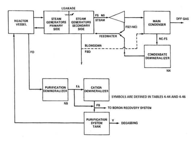
Figure 4-4 Removal paths for the reference PWR with U-tube generators
