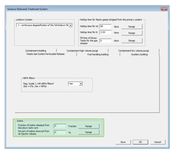
Figure 3-59 Gaseous Radwaste Treatment System Screen with Iodine field
