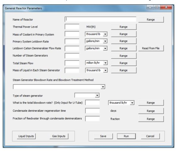
Figure 3-6 General Reactor Parameters Screen
