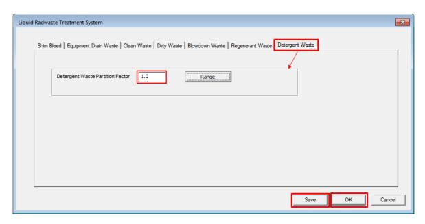
Figure 3-51 Liquid Radwaste Treatment System Screen (Detergent Waste Tab)
