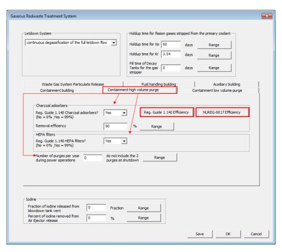
Figure 3-74 Gaseous Radwaste Treatment System Screen with Containment High Volume Purge Tab options
