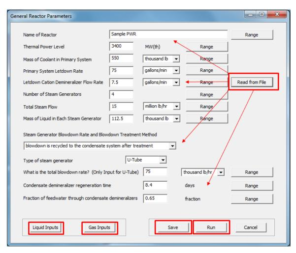
Figure 3-8 General Reactor Parameters Screen with default values from the PWRGALE.in file
