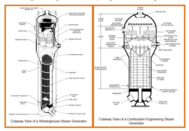
Figure 3-18 Cutaway views of Westinghouse and Combustion Engineering U-tube steam generators
