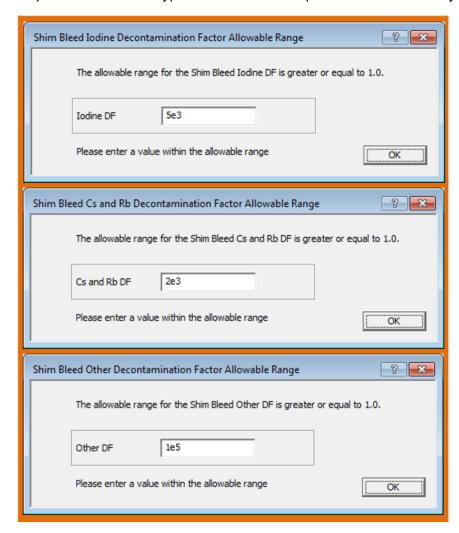
Figure 3-25 Shim Bleed Decontamination Factor Allowable Range Screens
