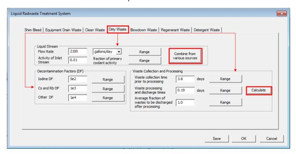
Figure 3-40 Liquid Radwaste Treatment System Screen (Dirty Waste Tab)
