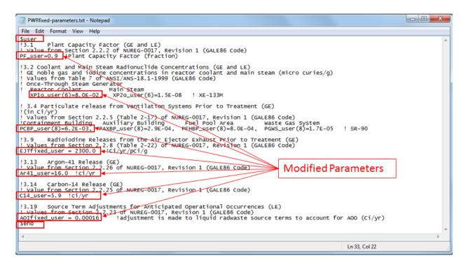
Figure 4-7 Example of a modified PWRfixed-parameters.txt file
