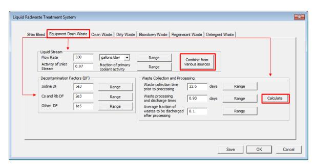
Figure 3-30 Liquid Radwaste Treatment System Screen (Equipment Drain Waste Tab)
