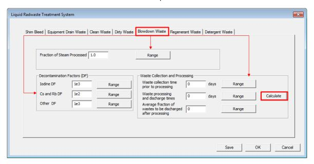
Figure 3-45 Liquid Radwaste Treatment System Screen (Blowdown Waste Tab)
