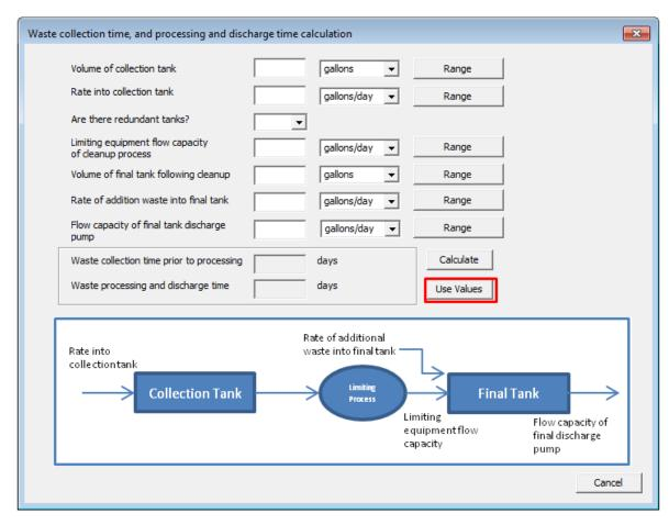
Figure 3-27 Waste Collection Time, and Processing and Discharge Time Calculation Screen
