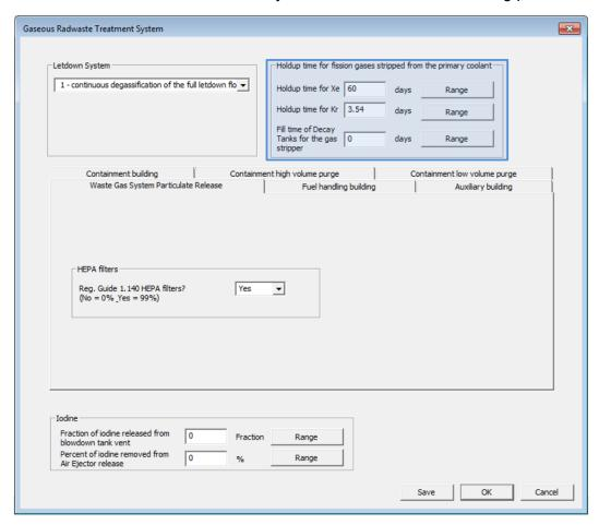
Figure 3-55 Gaseous Radwaste Treatment System Screen with holdup time for fission gases stripped from the primary coolant field
