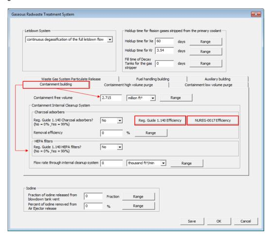
Figure 3-70 Gaseous Radwaste Treatment System Screen with Containment Building Tab options
