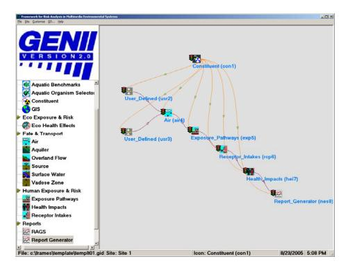
4<sup>th</sup> – The selected template will appear on the FRAMES screen. All module connections and model selections are now made; this is indicated on the screen as a series of icons, connected with colored lines, as shown below. It is recommended that the file now be saved using the FRAMES *File \ Save As* command; the user should assign a new name to the file so that the *Template* is not inadvertently overwritten.
