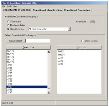
To complete the radionuclide selection, *left click* the *File* command and select *Save and Exit*. The window will close, and the contaminant icon on the FRAMES screen will now show a green "signal light" indicating that the data selection is complete.
