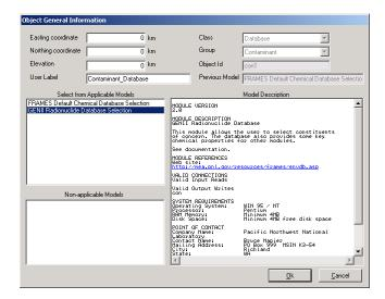
When the model has been selected, LEFT click on the OK button and the active window will return to the FRAMES workspace. If the model was selected correctly, the status light will be red.
