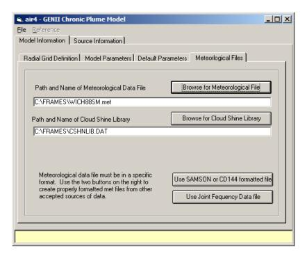
Use the *Browse for Meteorological File* button, highlight the desired file, and click on *Open* to select the input data. Sample files supplied with GENII end with the extension \*.met. Then right click on *File \Save and Exit*. The Atmospheric transport icon should now show a yellow "signal light".
