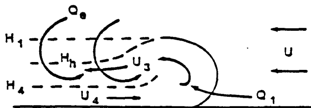
Figure V.4. The Head of a Steady Gravity Current (Simpson and Britter, 1979; van Ulden, 1983).
