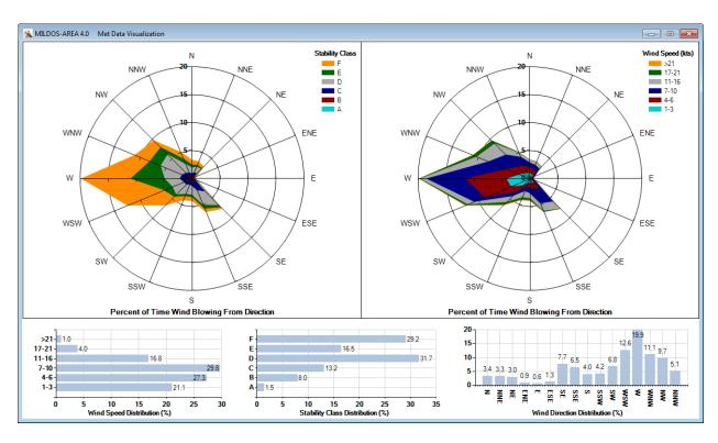
Figure 6-11 Graphic Presentation of the Meteorological Joint Frequency Distribution Data
