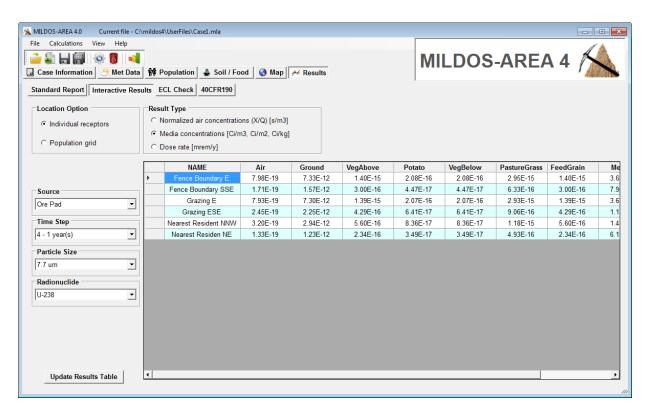
Figure 7-3 "Interactive Results" Output Tab Shown with Media Concentration Output Selected
