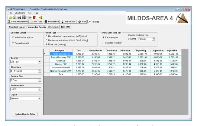
Figure 7-4 "Interactive Results" Output Tab Shown with Dose Output Selected
