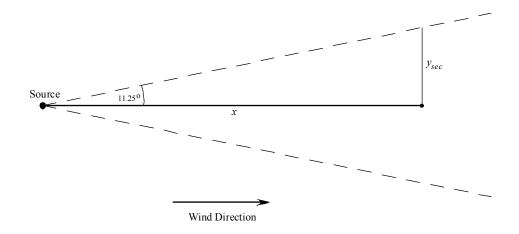
Figure 3-1 Relationships Used in Sector-Average Air Concentration Calculations
