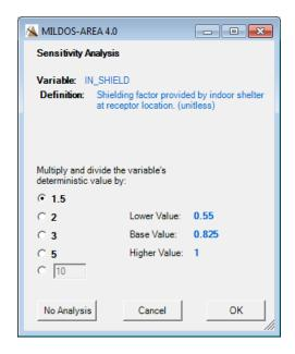
Figure 6-18 Sensitivity Analysis Input Form
