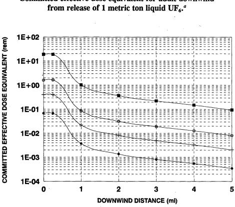
Fig. E-4 Committed effective dose equivalent for adult downwind from release of 1 metric ton liquid  $UF_{c_1}^a$
