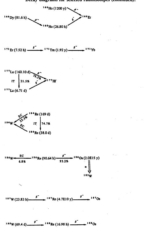
Fig. M-1 Decay diagrams for selected radioisotopes (continued).
