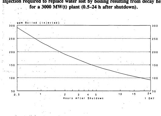
Fig. A-1 Injection required to replace water lost by boiling resulting from decay heat for a 3000 MW(t) plant (0.5-24 h after shutdown).
