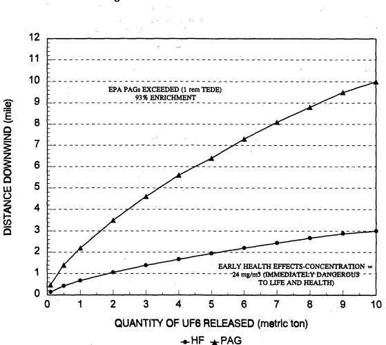
Fig. E-1 Distance downwind at which early health effects from HF exposure might occur or EPA PAGs could be exceeded.
