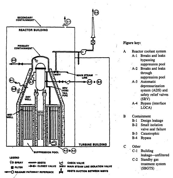
Fig. C-4 BWR Mark II simplified release pathways.
