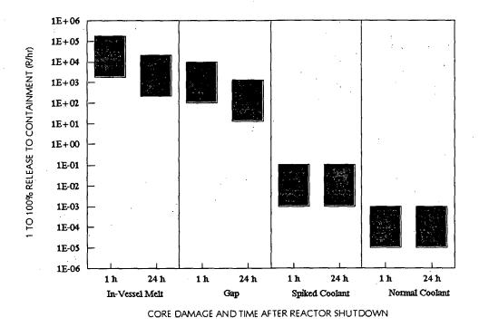
Fig. A-9 BWR Mark I & II wetwell containment monitor response.
