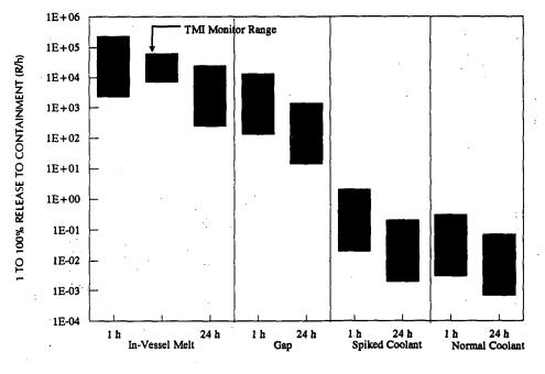
Fig. A-5 PWR containment monitor response (sprays on).
