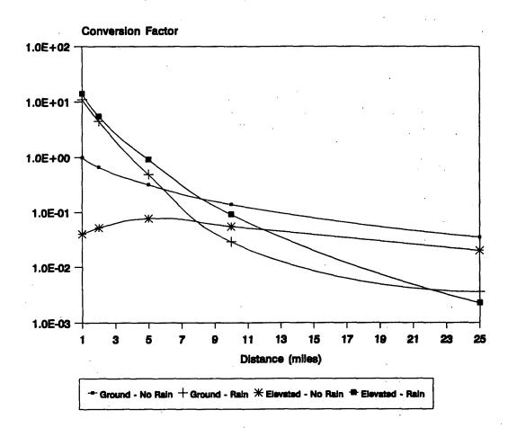
Fig. F-2 Conversion factors needed to adjust thyroid dose at 1 mile resulting from inhalation of plume for other distances and other release conditions.
