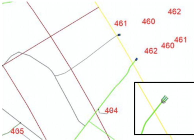
Figure 3-4 Illustration of Pitch-Fork Modeling Approach for Destination Zones
