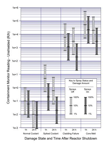
The model uses tables such as this one to convert the reading into a damage amount.
