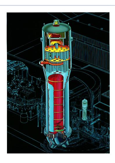
Each steam generator contains 3,000 – 16,000 tubes; each about 0.75 inches in diameter.
