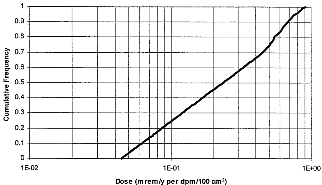
Figure 5.13 Calculated distribution of dose to the average member of the screening group due to a unit source of Th-230
